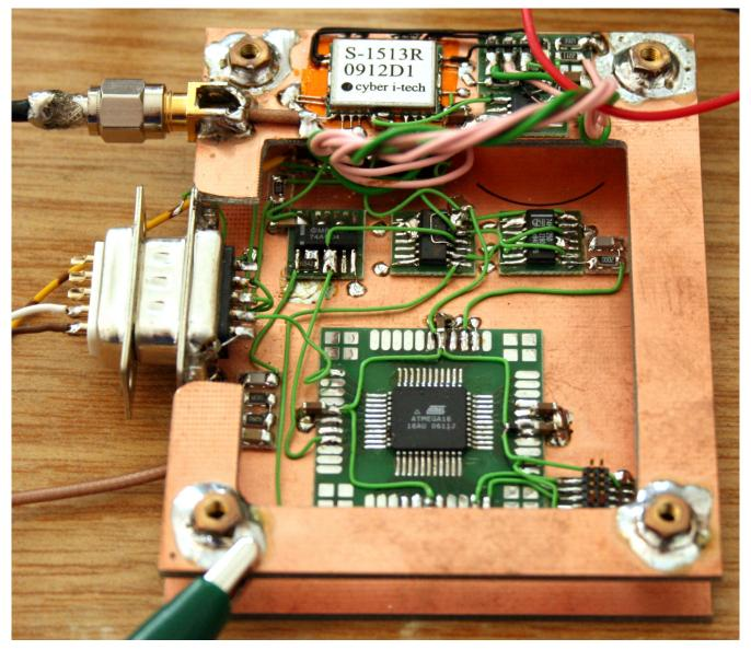
From left to right: GPS antenna input and RF Solutions GPS-1513R. This is a ROM Venus6 receiver. It is sitting on top of two layers of Kapton tape. Next to that is stupidity protection, and 3.3V regulator.
