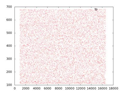
through the flipflop where it otherwise would not. This leads to a nonlinearity in the timedifference to analog conversion. For the case of an AC04 providing the clock, and an HCT04 providing the input signal to a HC74, the tp span should be 2,3% larger than it is, at 14.7456MHz clock.
