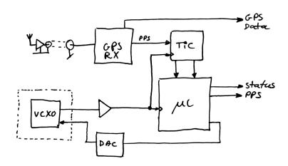
The GPS receiver delivers a time mark pulse, and we need to timestamp it against the reference oscillator. Since the cpu in the GPS and the cpu we use are likely to run at comparable clock frequencies, we need to timestamp with better than 1 clock resolution. If we do not, we get twice the error, and we get funny interference effects which are hard to impossible to suppress in software.
