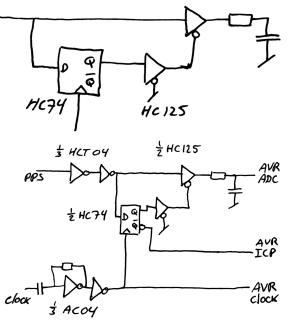
have at least a +/- 25 ns (@20MHz) window around the rising edge to get the ICP signal to the AVR so as to have it recognized in the correct clock cycle.
